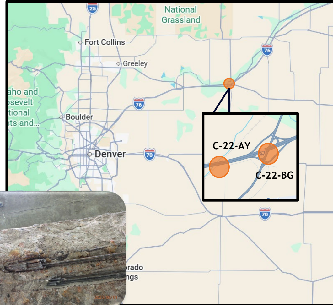
Broken PT strands in girder at C-22-AY
