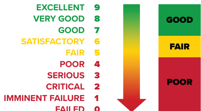
Figure A.10-3 Overall Wall Condition Rating Scale
