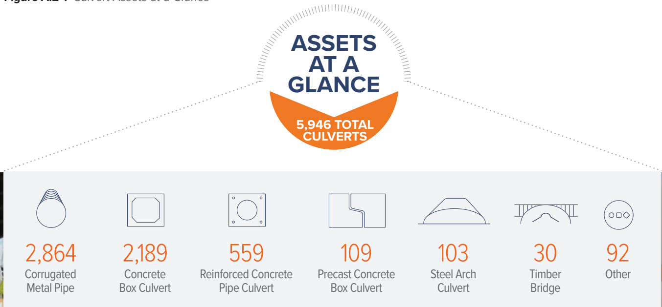
Figure A.2-1 Culvert Assets at a Glance
