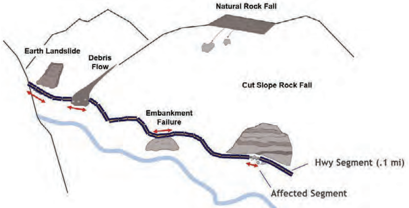
Figure A.4-1 Examples of Geohazard-Affected Segments
