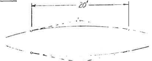
V.C. AT TOP OF WALL SLOPE CHANGE Where Shown on the Plans
