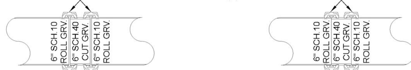
UN-EXPANDED PIPE (2) COUPLINGS AT MAX PARALLEL DEFLECTION EXPANDED PIPE (2) COUPLINGS AT ZERO PARALLEL DEFLECTION
