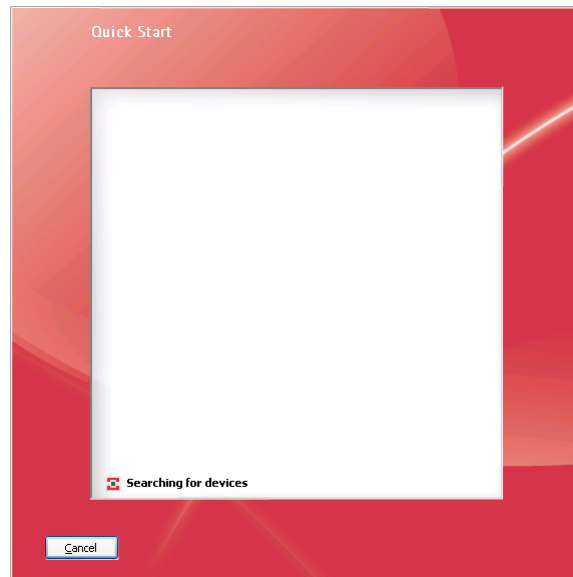
Figure 37: START window with message SEARCHING FOR DEVICES (being displayed if no controller is connected)
