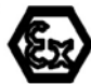
Figure 79: Printing Text detail – Marking example for ATEX and IEC Ex approved I/O modules according to CENELEC and IEC
