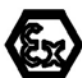
Figure 17: Printing Text detail – Marking example for ATEX and IEC Ex approved I/O modules according to CENELEC and IEC
