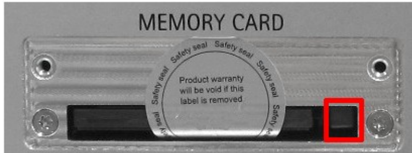
Figure 59: Open memory card slot with safety seal on the CF memory card and eject pin (marked by the red square)
