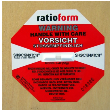
Figure 13: Shock label. A red tube in the centre would indicate rough handling
