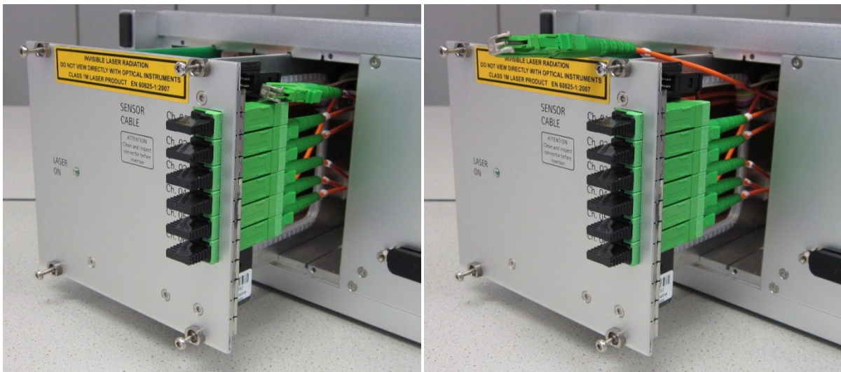
Figure 56: E2000 connector removed from the mating adapter (left) and slightly drawn out of the enclosure (right).
