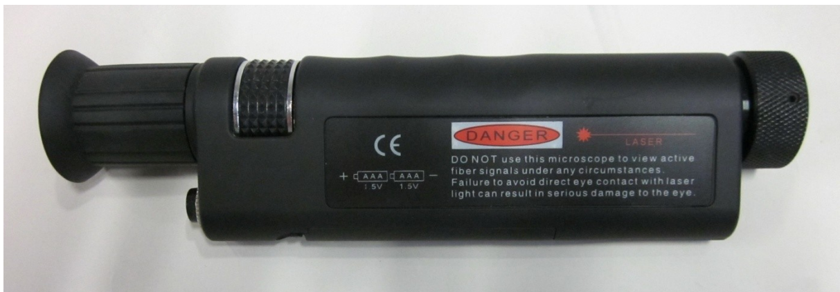
Figure 34: Fibre scope with 200x magnification, built-in laser filter and LED illumination
