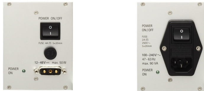
Figure 10: DC (left) and AC (right) power supply panels
