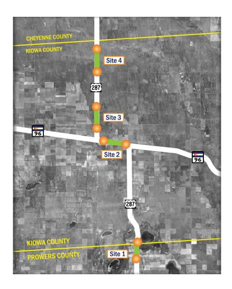
Two northbound passing lanes were added to US 287 between exits 94 and 96 to exits 114 to 116. Two southbound passing lanes were added between exits 110.9 to 112.4 and exits 120 to 122.
