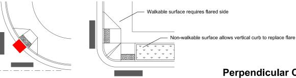
Perpendicular Curb Ramp As-Built Form (Sheet 2 of 2)
