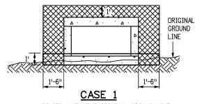
APPLIES WHEN THE ORIGINAL GROUND LINE IS LESS THEN 1 FT. ABOVE THE BOTTOM OF THE BOX CULVERT. THE EMBANKMENT SHALL BE BUILT UP TO 1 FT. ABOVE THE BOTTOM OF THE BOX CULVERT AND THEN EXCAVATED TO THE BOTTOM OF THE BOX CULVERT. THIS EMBANKMENT AND EXCAVATION WILL NOT BE MEASURED AND PAID FOR SEPARATELY BUT SHALL BE INCLUDED IN THE COST OF THE WORK.
