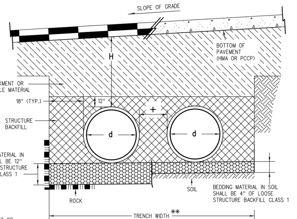
**INSTALLATION OF MULTIPLE PIPES**
