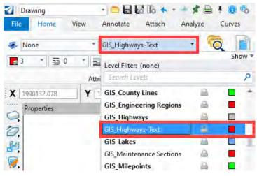
13. Turn off all the levels not being labeled except for the level to be annotated and no plot level. The illustration below shows the levels used in the example.
