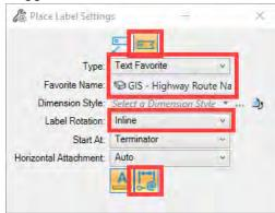
20. **Left Click** on the element to be annotated near where the label is to be placed. Move the cursor to rotate the label to the desired direction then **Left Click** to place the label.
