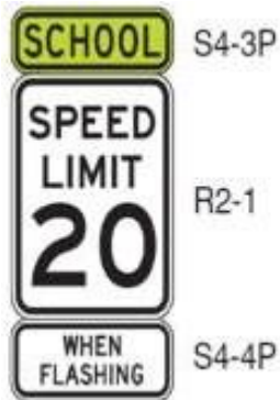
Figure 13-71 School Speed Limit Assembly
