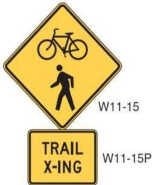
Figure 13-50 Trail Crossing Assembly
