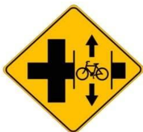
Figure 13-58 Example Adjacent Path Sign
