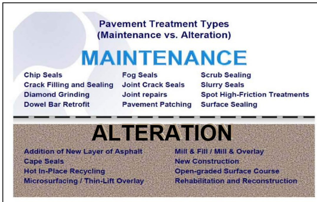
Figure 12-1 Maintenance vs. Alteration for Surface Treatment Projects
