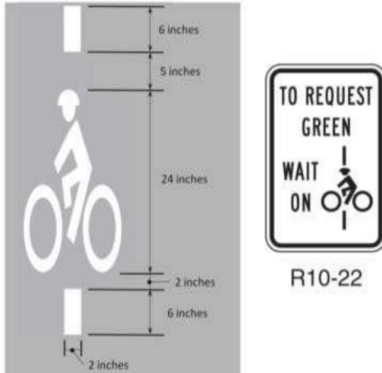
Figure 13-33 Bike Detection Symbol and Bicycle Signal Actuation Sign
