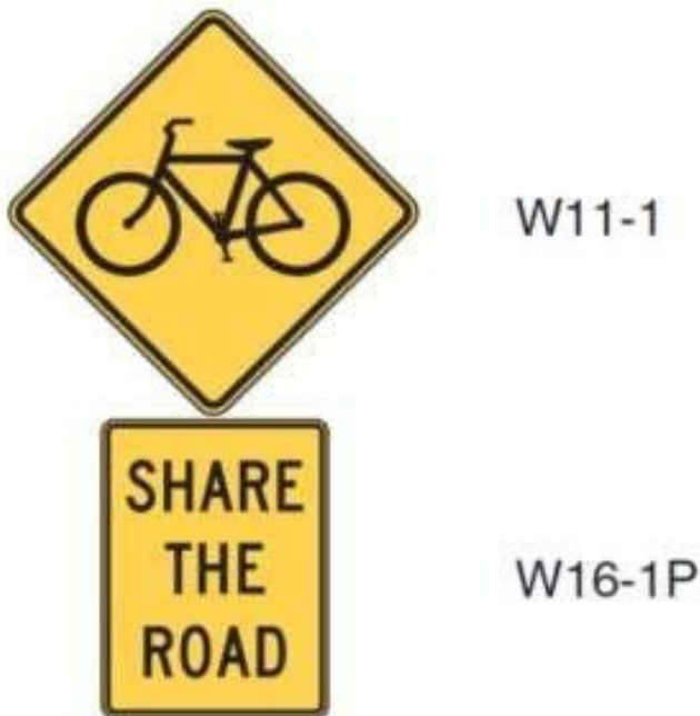
Figure 13-11 Share the Road Sign Assembly
