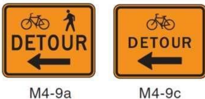
Figure 13-59 Bicycle Facility Detour Signs
