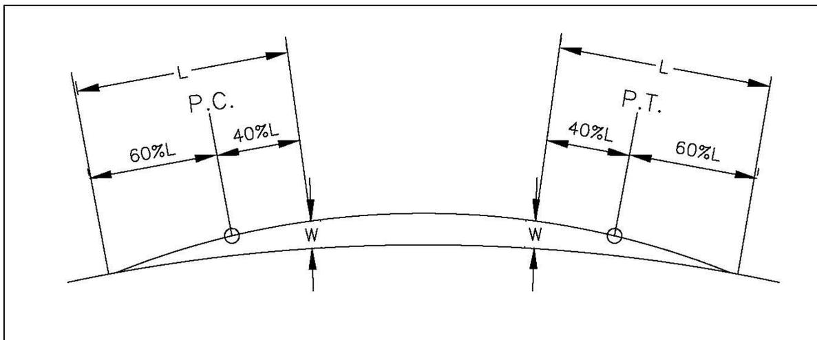
Figure 3-12 Widening on a Simple Curve
