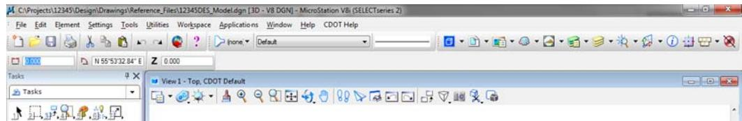
**Note:** Any toolbar can be docked on the perimeter (top, bottom, left, or right sides) of MicroStation's application window.
