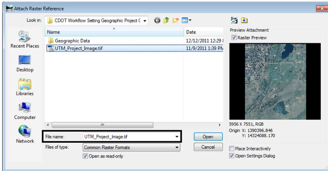
In this example, the image is from a portion of Colorado where the coordinate system is UTM. These files are GeoTIFF files with the coordinate system written into the header of the file. There is no sister file accompanying the image.
