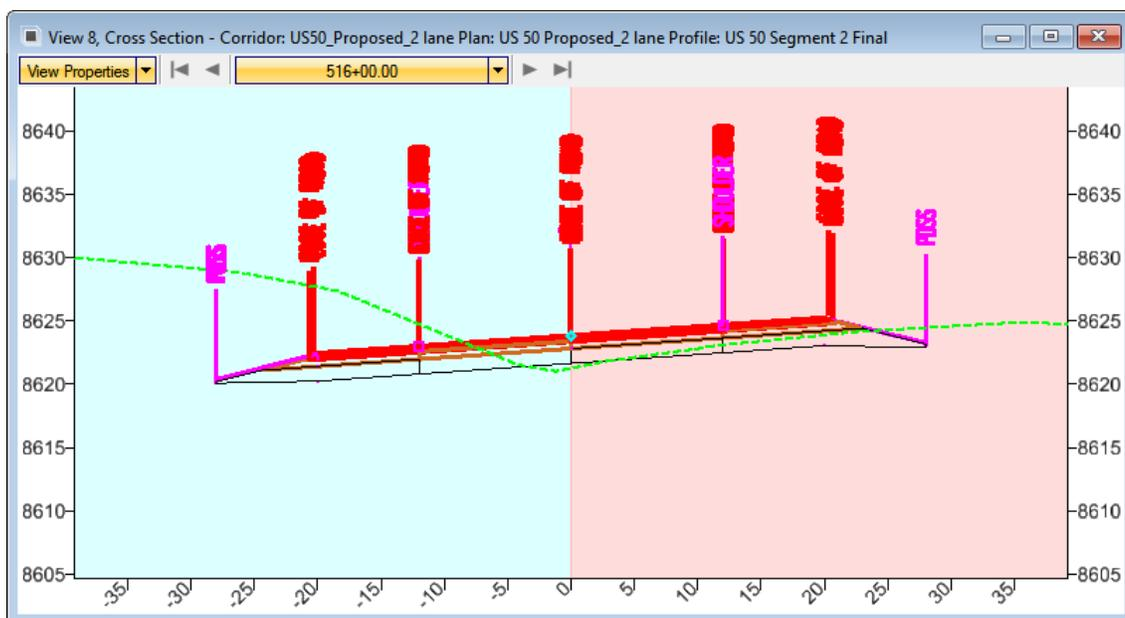
**Note:** Missing end conditions are caused by Target Aliases to design surfaces. These Target Aliases will be rebuilt to use the corridor. This is explained in Section V below.
