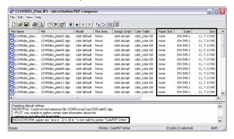
34. To correct this problem you will need to change the active printer and change the paper size setting. Select File > Form Setup... from the pull-down. This will display the Form Setup dialog. From the list of available printers select a printer that supports your paper size setting, then <D> OK.
