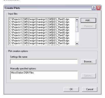
6. After reading in each of the dgn files the MicroStation PDF Composer window will display with all of the sheets listed. The plot area(s) for each file are automatically extracted by reading the shape element limits on the SHEET\_Plot-Boundary level. PDF Composer will generate multiple plots from a single file if more than one shape is found on the plot sheet boundary level. The other automatic setting you will notice is to scale the output for tabloid (11x17) paper size.
