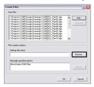
31. Select the settings file that matches your required paper size and rendering. Listed below are the general equivalent MicroStation pen table files to assist with making the right selection:
