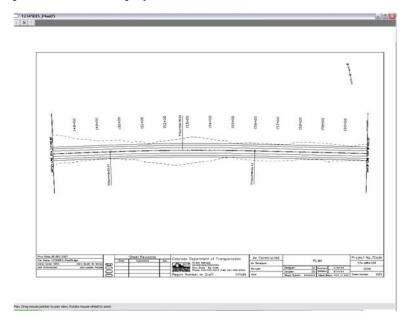
21. If multiple sheets were selected for preview you may navigate between the sheets by using the forward and back arrows in the top left corner of the preview window. Measurement functions and windowing functions such as **Zoom**, **Pan**, and **Fit** are available via a right click menu. <R> anywhere within the preview window to display this menu.
