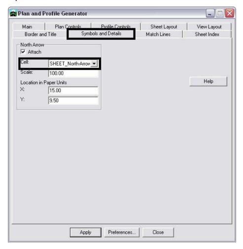
The *North Arrow* position is specified by the Location in Paper Units input and is set to the upper right corner of the sheet. This is a rough placement and will likely have to be moved for clarity and conflicts on many sheets. Once the sheets are constructed each sheet should be checked for optimum cell position.
