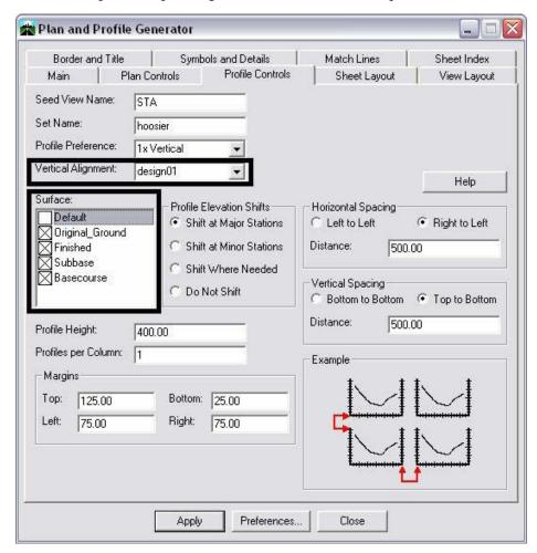
Profile Preference defines profile grid settings (ticks, annotation, grid/tick spacing etc.) as stored as a preference in Evaluation > Profile > Generate Profile
