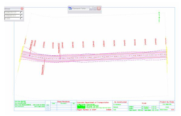
The graphics in a sheet file represent only a portion of the entire design and are usually included within a standard border. The image above is a portion of the graphic representing the design file on the previous page.
