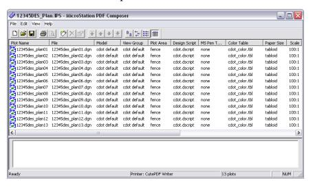
3. To recreate the PDF file select File > Export PDF... from the MicroStation PDF Composer pull-down as before and repeat Basic PDF Composer Workflow steps 6-15. The new PDF file will reflect changes made to the MicroStation design files as well as any changes in the referenced Design Script(s).
