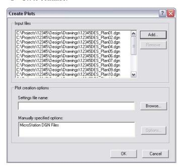
After reading in each of the dgn files the *MicroStation PDF Composer* window will display all of the sheets selected. The plot area(s) for each file are automatically extracted by reading the shape element limits on the *SHEET\_Plot-Boundary* level. PDF Composer will generate multiple plots from a single file if more than one shape is found on the plot sheet boundary level. The other automatic setting you will notice is to scale the output for tabloid (11x17) paper size.
