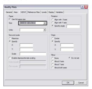
Note: As you can see from the figure above there are many other plot settings that can be modified. When applying the correct settings file in combination with the appropriate active printer these other settings will rarely need to be modified. Setting the correct *Paper Size* will change the *Scale* and *Size* settings to the correct values.
