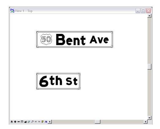
Note: SignCAD places the graphics on the Default Level and at an Elevation other than zero (Z=0). You will need to select the graphics and change them to the correct MicroStation level (*TRAF\_SIGNING\_Proposed*). You can use the *MOD Z* utility from Add On's > ModZ found on the *CDOT Menu* to change the elevation to zero (Z=0).
