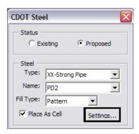
The CDOT Steel Settings dialog allows for adjusting placement scale and rotation values as well as the placement justification for each section type.
