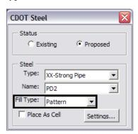
5. The steel components can be placed as cell elements by selecting the *Place As Cell* checkbox. When placed as a cell the cell name is set to the value in the *Name* drop-down.
