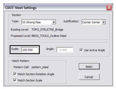
5. To change the placement angle to something other than the active angle setting uncheck the *Use Active Angle* checkbox and enter a new rotation angle.
