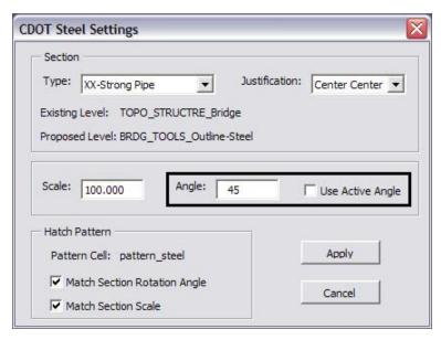
6. To vary the hatch pattern angle and/or scale independently of the section values, uncheck the appropriate *Match Section* checkboxes. With these boxes unchecked, patterning will use the active design file settings.
