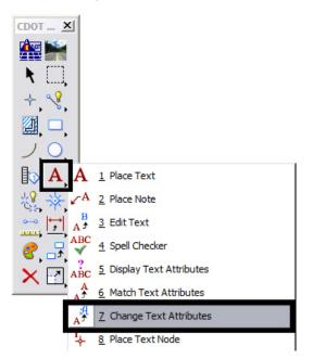
In the Change Text Attributes dialog box, set the Text Style. Use .10" ENG-100 Filled for Major Stations and .07" ENG—100 Filled for PC, PT, and PI stationing Points. Also, set the desired Justification.
