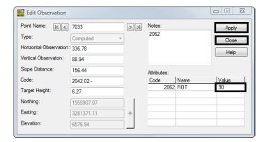
52. **<D>** the **Apply** then **Close** buttons. The end section cell will have rotated into the direction of the pipe.
