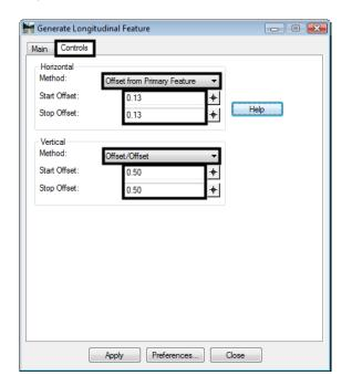
49. Key in **0.50** for the **Start Offset** and **Stop Offset**. This is the height of the curb.
