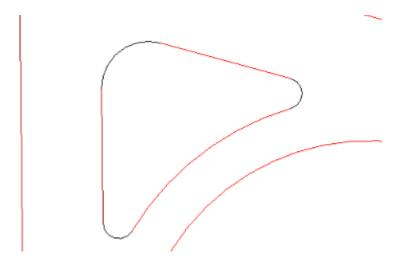
With the outline of the island in place, the pedestrain ramps can be located. These are placed in the center of each side of the island. The MicroStation Construct Line At Active Angle command is used to place the ramp centerline perpendicular to the island side.
