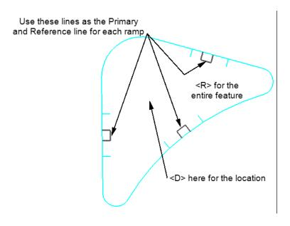
39. Repeat step 38 for each ramp. The illustration below shows the results. Dismiss the *Generate Longitudinal Feature* dialog box when finished.
