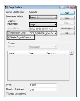
7. **<D> Apply**. This displays a message window asking, "Use elements contained in selection set?". **<D> OK** to complete the processing.
