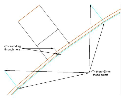
This has broken each of the curb top lines into four sections. The sections inside the ramp area will be modified after they are imported into the surface. Those outside will be left as is.
