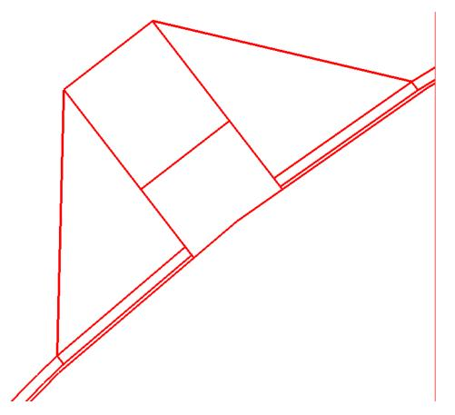
In a rotated view, notice that the curb top lines do not slope consistantly from the wing to the tread. This is because the Trim Feature command matches the elevation from the intersection of the features to the next vertex in the trimmed feature.
