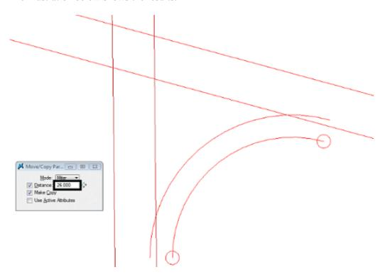
Next the radii for the island corners are added. The corner facing into the intersection has a 15' radius. The other two have a radius of 5'. These are placed using the Construct Circular Fillet command.
