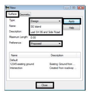
This surface is used to store the island surface data as its being created. It also protects the data in the Intersection.dtm from being accidently modified while editing the island surface features.
