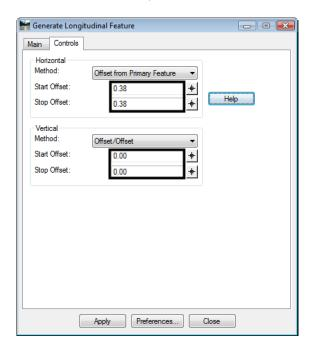
54. **<D> Apply**. Then follow the prompts. **<D>** a top of curb element for the primary feature and use the same one for the reference feature. **<D>** in the middle of the Island for the location. The illustration shows an example of the results.
