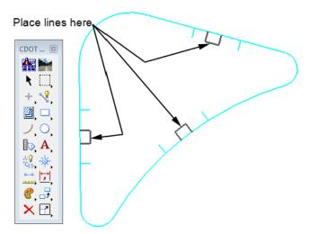
Next, the generate longitudinal feature command is used to create the back of the pedestrian ramps.
