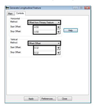
38. **<D> Apply**. Then follow the prompts. Use the ramp tread end line as the primary and reference element. **<R>** to use the entire line. **<D>** in the middle of the Island for the location.
