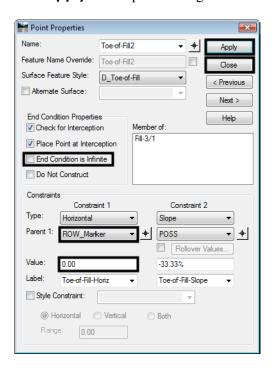
52. **D> Apply** to accept the changes. **D> Close** to dismiss the dialog box.
