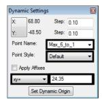
The <code>Max\_6\_to\_1</code> point is placed in the correct location, but it is not constrained. It should be constrained to the pavement edge sot that the proper distance is maintained if the pavement width is changed.
