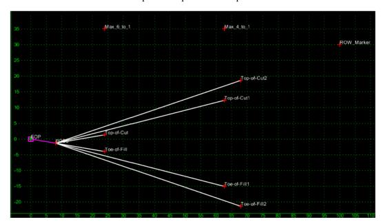
Next, the constraints on the toe points are changed to use the three Null points just added.
