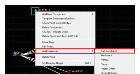
18. <R> on the *Max\_6\_to\_1* point and select Add Constraint > Full Constraint from the right click menu.
