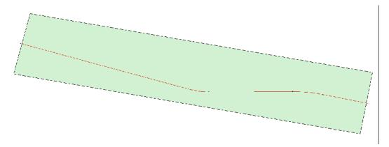
Next, a feature filter is set up that will only display edge of pavement features. In this case these features are named T-Edge of Oil.
