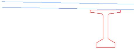
This places the first girder 3 ft. – 6 in. from the right side of the slab. You'll later move the girder down for the proper haunch depth.
