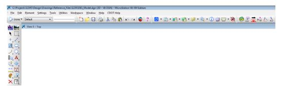
**Note:** Any toolbar can be docked on the perimeter (top, bottom, left, or right sides) of MicroStation's application window.
