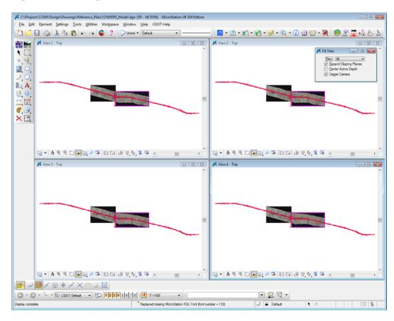
5. Repeat the above steps to rotate views 3 and 4 to a **Top** view and **Fit** the views.
