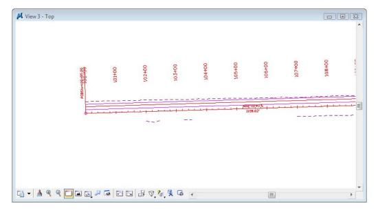
4. While still in the **Window Area command**, move your cursor over to View 4 and **<D>** above and to the left of the alignment end as shown.
