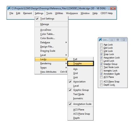
**Note:** A settings box, like the Locks box, does not have any command buttons (**OK**, **Close**, etc.). Settings boxes can be left open while working in MicroStation.
