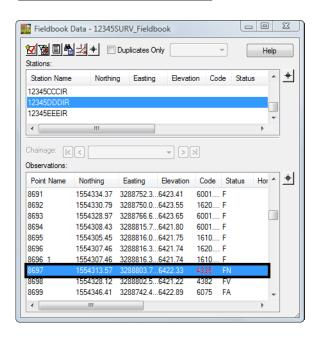
**Note:** This error has an incorrect Feature Code for a power pole.
