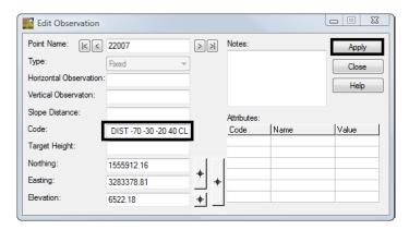
**Note:** A *positive number* will place the line to the *right* of the two base line points. A *negative number* will place the line to the *left side* of the two base line points.
