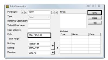
**Note:** A positive number will place the rectangle on the right side of the two base line points. A negative number will place the rectangle on the left side of the two base line points.
