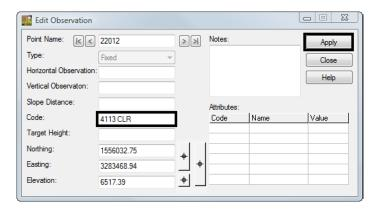
25. **<D>** the **Apply** button the close rectangle control code will have finished creating the line work.
