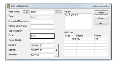
24. **<D>** the **Apply** then Close buttons. In the MicroStation View 1 the point has been updated and a power pole cell is at the location.
