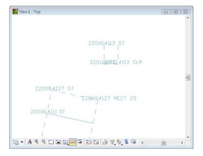
The watermain and a hydrant have been surveyed The control code JNC will be utilized to tie the hydant to the watermain.
