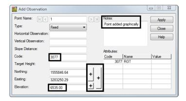
8. **<D>** the **Apply** then Close buttons. The tree will dynamically display in the MicroStation view.
