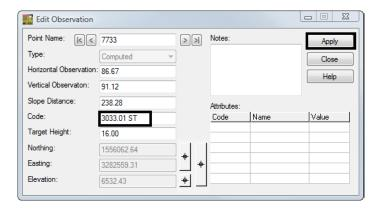
59. **<D>** the **Apply** then Close buttons. The change in direction for the feature code will correct the planimetric display.
