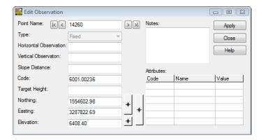
23. **<D>** the **Target** button. The *Edit Observation* dialog will minimize allowing to select a point in the MicroStation view.
