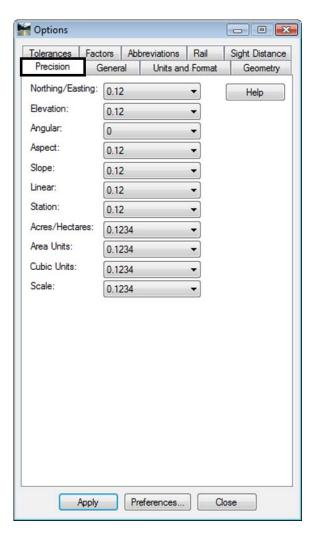
The *precision* tab defines the number of decimal places displayed in dialogs. It also defines the number of decimal places displayed when posting information to the MicroStation screen or when writing data to an ASCII file.
