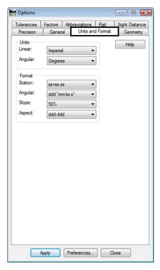
InRoads does not recognize or use the unit definition associated with the host MicroStation file. The units defined under the *units and format* tab define the units of measure for InRoads data. For commands that utilize distance or area parameters, InRoads looks to the settings in this dialog to determine if the distance or area defined is imperial or metric units.
