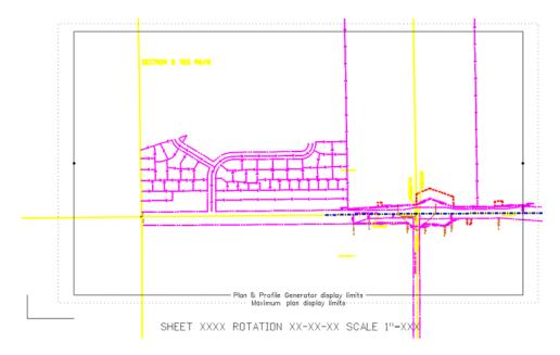
The above graphics approximately represent the required limits for the first sheet. Position the sheet limit cell as you see fit.
