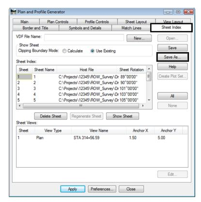
The Sheet Index tab will display a list of sheets created and MicroStation will display the last sheet created.
