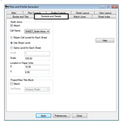
The **North Arrow** position set by the **Location in Paper Units** and is set to the upper right corner of the sheet. This is a rough placement and will likely have to be moved for clarity and conflicts on many sheets. Once the sheets are constructed each sheet should be checked for optimum cell position.
