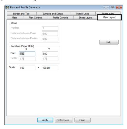
**Note:** The Location of the Plan position is computed from the outside edge of the border sheet in paper (plotted) units.
