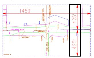
**Width Left** and **Width Right** define plan view limits perpendicular from the reference line (left is negative).
