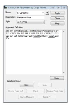
**Note:** The alignment C\_Centerline is defined as having Cogo point numbers assigned at its vertices. The letter C indicates the Cogo point identified is the Center of a curve. The letters R or L indicate the curve direction (Right or Left).
