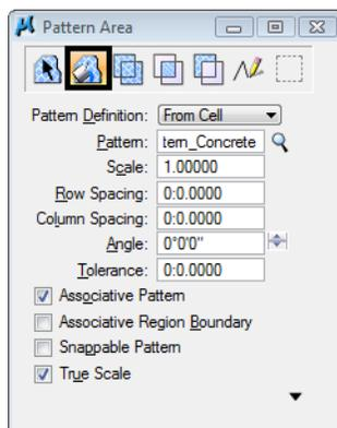
4. Make sure the entire region to flood is shown in your view. Then, <D> anywhere inside the bridge slab region. The region to flood with the pattern highlights.
