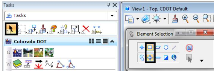
2. Place a fence around the slab graphics (<D> for upper left corner and then <D> for lower right corner).
