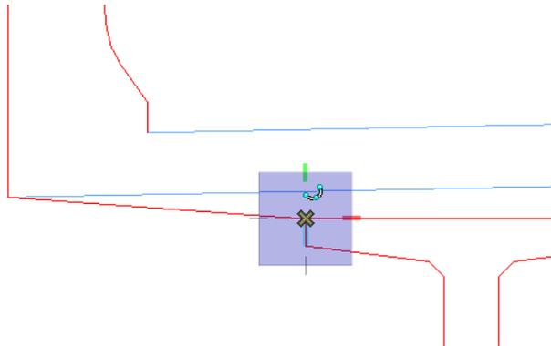
6. Move your cursor down, lock on the **Y** axis and key in a value of **:1** (1 inch).
