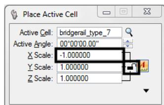
**Note:** **-1** X-axis scale will mirror the cell about the X axis.
