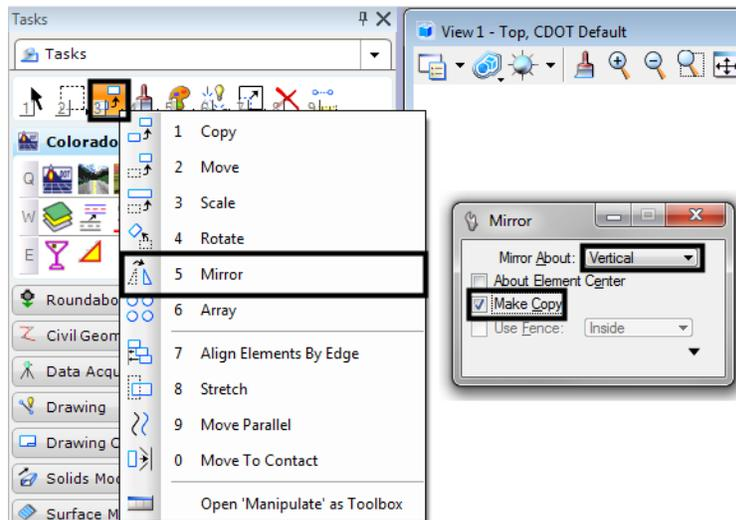
4. <D> on the left endpoint of the upper slab line (the crown point) for the mirror copy.
