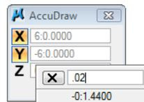
14. <D> to place the second **SmartLine** segment, this creates the 6 ft. shoulder at a 2% slope.
