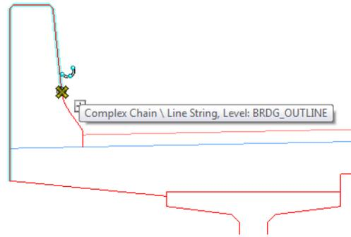
8. Select the **Copy** command from the **Primary** toolbar and copy the bridge rail to a clear area of the design file.
