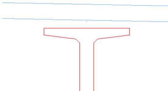
This moves the girder down 4 inches from the bottom of the slab for the correct haunch thickness.
