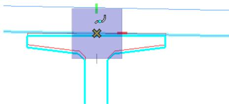
8. Move your cursor down to establish the move direction, lock on to the **-Y** axis and key in **:4** in the **AccuDraw Y** field.
