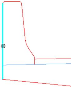
5. <D> anywhere above this element to define the direction for adding elements. The remaining bridge rail elements are added to the chain and placed on the active **Bridge\_Outline** level.
