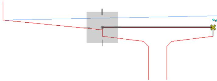
10. Move your cursor up, lock on to the **Y** axis and press **<Enter>** to smartlock the axis. You can now only move in the **Y** direction.
