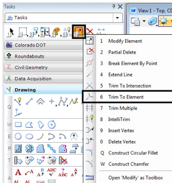
25. <D> on the blue top of slab line and then <D> on the back of bridge rail line to extend these elements.
