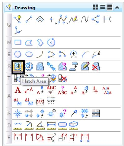
7. In **Tool Settings**, select the **Flood** method, set **Spacing** to **:3** and the **Angle** to **45**.
