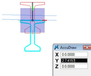
By pressing <Enter> you “smartlock” the **AccuDraw X** and **Z** axes, so that you can only move in the **Y** direction.
