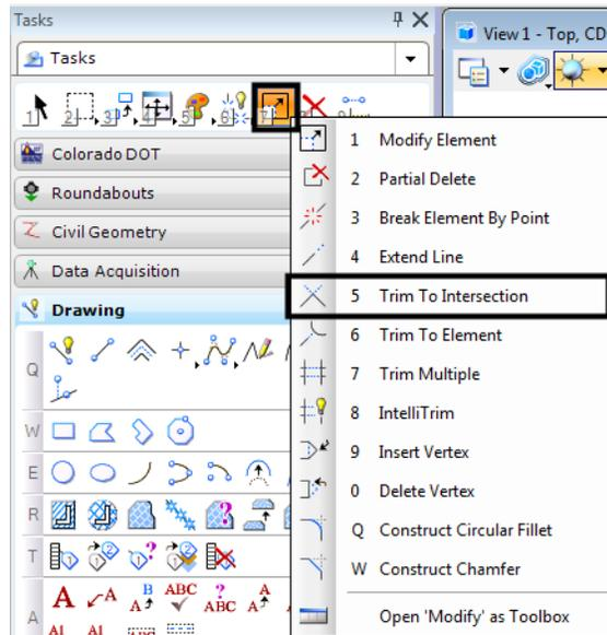
6. <D> on the bottom slab line and then <D> on the back of rail line to extend these elements.
