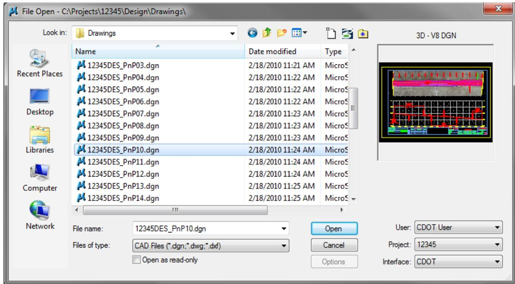
The **InRoads Plan/Profile Generator** automates the creation of sheet files along the mainline alignment. This includes rotating the plan-view to horizontal, placing the corresponding profile, placing the border, north arrow and match lines. MicroStation references are used to bring in plan and profile graphics to the active sheet file.
