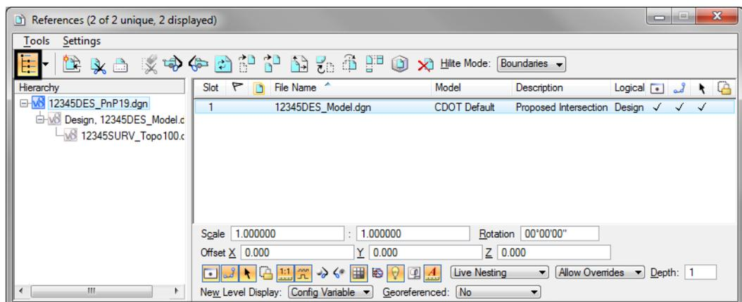
**Note:** Note that with nested references, the Survey/Topo reference is nested below the Design model file. You can typically reference model files as nested to sheet files instead of using the **Copy Attachment** command (as in this case, you want to show both Design and Survey/Topo graphics in the sheet file). However, if you need to control individual references in the sheet file, then use the **Copy Attachment** command.
