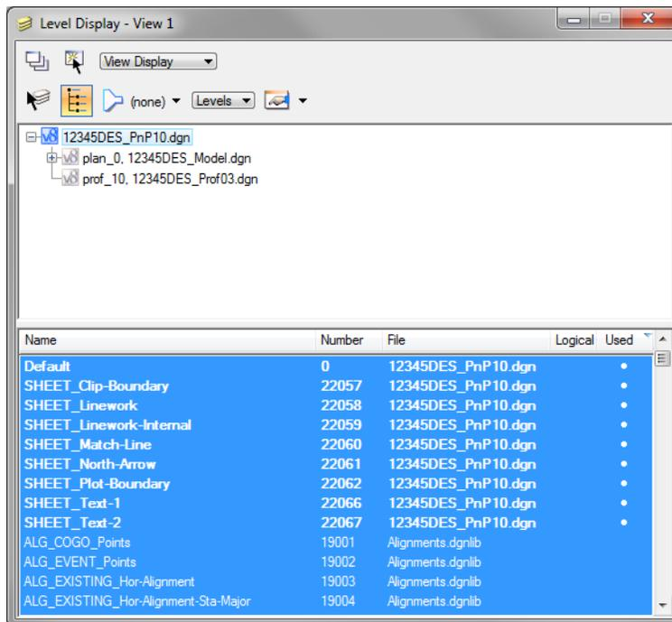
**Note:** Only levels with graphics in the sheet file are sheet levels for the border, match line, north arrow, *etc.*
