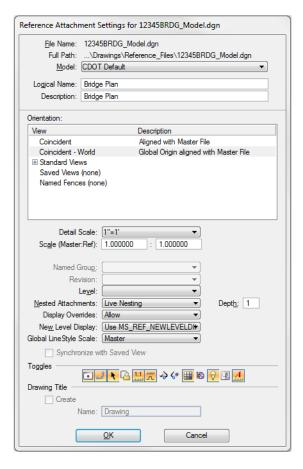
The bridge plan and the nested design reference are attached to the sheet file. Since you attached at a 1:1 scale and Coincident-World, all of the bridge plan graphics are in their true coordinate locations and actual size.
