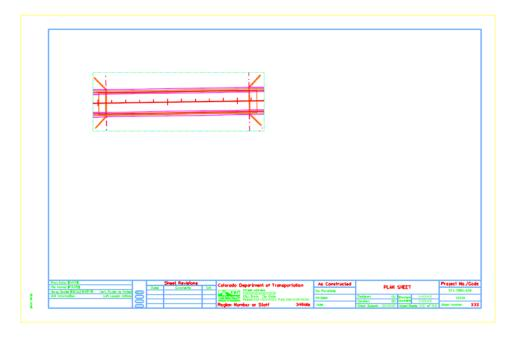
The bridge plan is now place inside the border at the proper coordinates. Design graphics levels can be turned on/off as needed.
