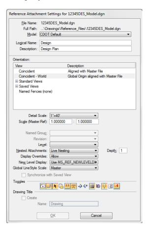
The design model is attached coincident to the proposed bridge graphics. A nested depth of 1 also references the Survey/Topo file (currently the Survey/Topo display is off). You will later reference the bridge plan to a sheet file.
