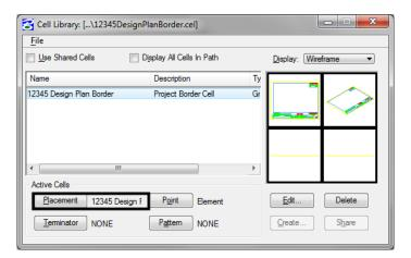
4. Select the Place Active Cell command and place the border at a 40 scale.
