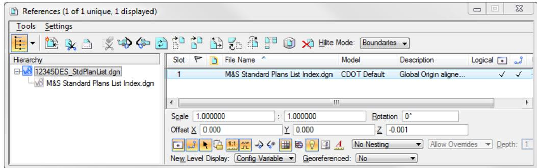
Note that the M&S StandardPlansListIndex.dgn file is already referenced from the project’s \Design\Drawings folder. It was automatically placed here from the Create Project Directory utility.
