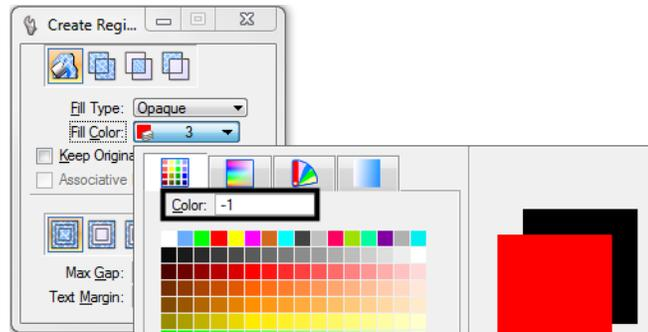
**Note:** If the Fill Color is set to By Level, the Tool Settings dialog box will not be updated if the active level is changed. However, the color of the new active level will be used when the region is created.
