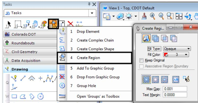
**Note:** The Fill Color drop down shows the color number assigned to that level when it is set to By Level. To check if it set to By Level, <D> **Fill Color** drop down. If the Color field reads “-1”, then it is set to By Level.
