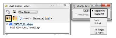
Turn *on* all of the alignment levels (data point <D> and drag across all ALG levels.
