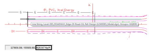
The edge of oil line is placed at the correct elevation.
