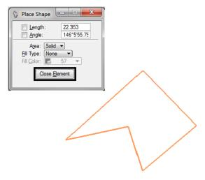
17. In the Tool Settings box, set Fill Type to Opaque and place another shape.
