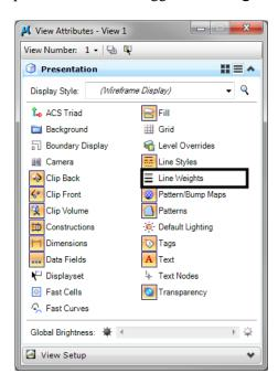
**Note:** Selecting the down arrow from the view attributes icon box temporarily allowing the user to toggle on line weights without bringing up the dialog box permanently. The dialog box will disappear when the mouse if moved away.
