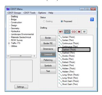
11. Place another **SmartLine** and note the change in line style and the active level on which it is placed.
