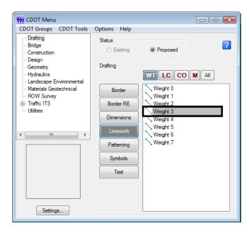
The filter determines the appropriate drafting level for the **SmartLine**. The Smartline command is the default for this menu item. All other drafting commands should be either be picked from the CDOT Main tool bar or entered as a key-in.
