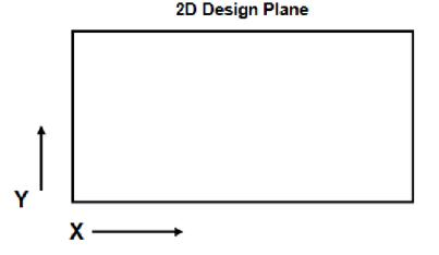
You can rotate the 2D design plane about its perpendicular axis (the Z axis coming out of the screen).
