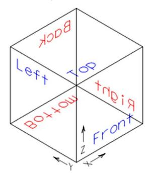
Think of a view as a camera location that's taking a snapshot of your design. When you rotate a view, you're **not** rotating **graphics**. Instead, you're rotating the camera position (or the orientation) of how you're looking at the graphics.
