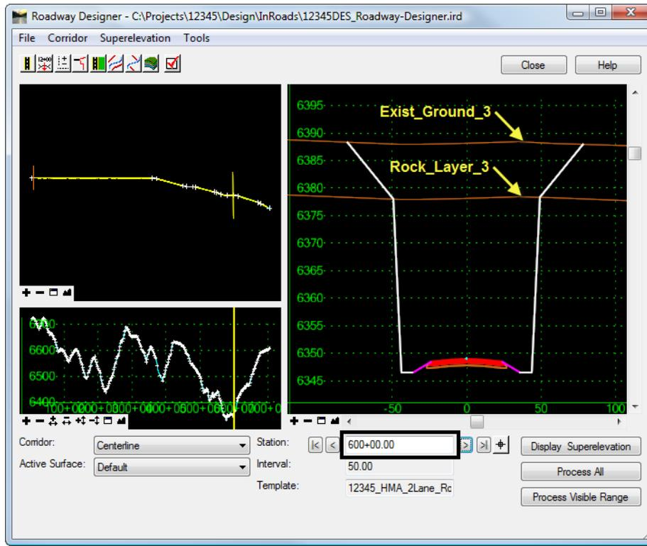
**Note:** Notice the end conditions target the multiple existing ground and rock layer surfaces in both of the above Roadway Designer dialog's cross-section viewer. Both of the station locations shown are in deep rock cut sections in the profile.
