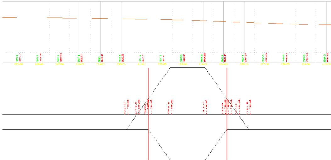
The green text (to the left of the grid line) represents the existing ground elevations. The red text (to the right of the grid line) is the proposed elevations. The super-elevation diagram is placed below the profile grid.
