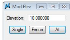
You can specify the elevation to planarize a single element, elements within a fence or all elements in the design file.
