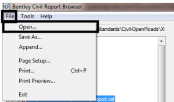
8. In the **Open** dialog box, navigate to the folder containing the desired IRD file. This will typically be the project's **Design\InRoads** folder.
