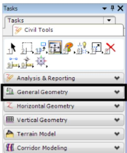
7. In the **General Geometry** tasks, left click the **Import Geometry** button. This displays the **Import Geometry** dialog box.
