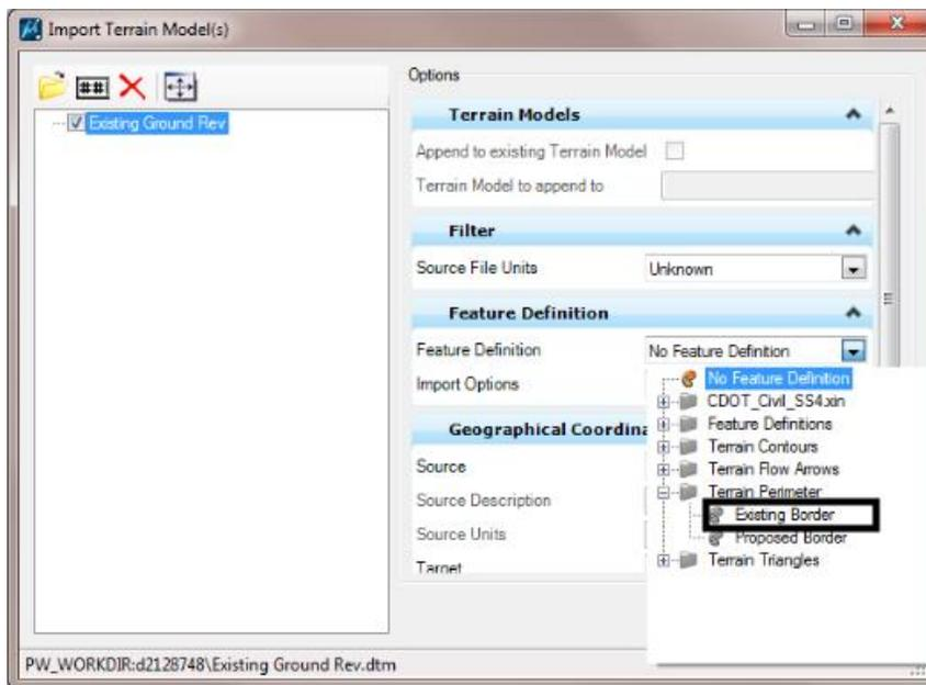
10. Set the **Import Option** to **Import Terrain Only**. This imports only the terrain model and not the Features. Triangles and break lines are automatically created as components of the terrain model element.
