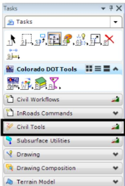
6. Under the **Civil Tools** task, expand the **General Geometry** task.
