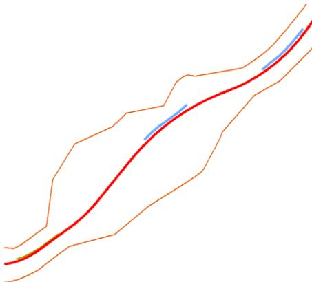
14. At this point, notice that there appears to be duplicate elements shown in the view. This is because the 3D model created by OpenRoads is automatically referenced to the 2D model. In **Reference Manager**, turn off the display of **Default 3D** for better clarity in the view.
