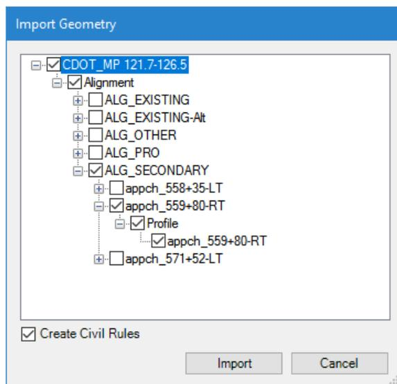
12. Select the horizontal and vertical alignments for the approach; **appch\_559+80-RT** in this example.
