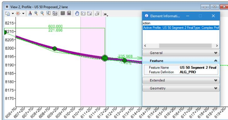
22. Notice that the **Name** and **Feature Definition** for the vertical alignment also match the ALG file.
