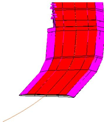
20. The density of the model is fairly sparse. This is a function of the design stage we chose, which purposely degrades the density for better performance. Later, the design stage can be changed to provide maximum density for the final model.
