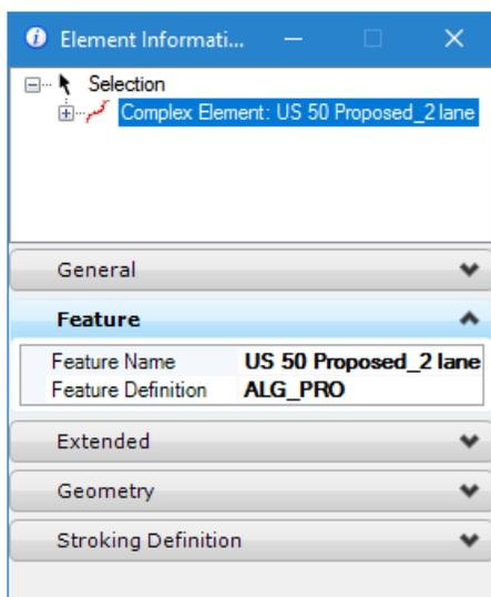
16. Note that the alignment name matches the name in the ALG file and the **Feature Definition** matches the style name used in the ALG file.
