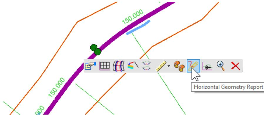
The report can be used to verify the import was successful. Also, a review of the start and end stations shows that the centerline length is about 3.7 miles long. This is fine for the alignment but we will want to be watchful after the corridor is imported to see if it performs well when editing and is stable. Generally, we will want to keep corridor lengths to less than 2 miles for best computer performance. We will keep this in mind when we get to the next section.
