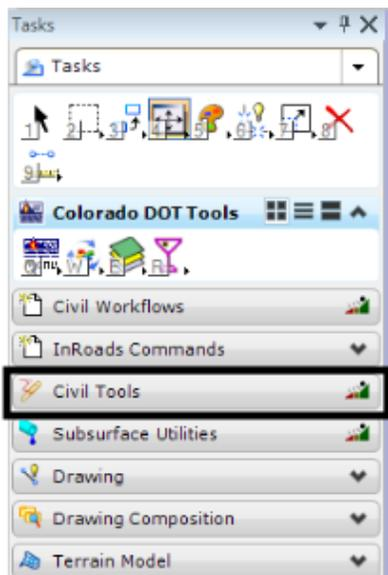
5. Under the **Civil Tools** task, expand the **Terrain Model** tasks.
