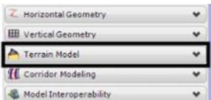
6. In the **Terrain Model** tasks, left click **Create from File** button. This displays the **Select Files To Import** dialog box.
