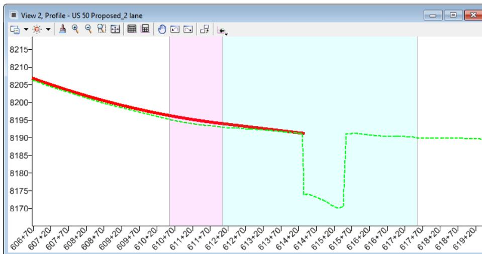
21. In the Profile View (**View 2** in this example), Select the vertical alignment element and **Open Element Information**.
