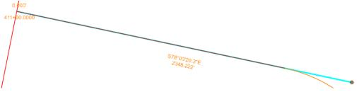
c. Change the bearing to N 70 00 00 E, note the alignment adjusts. Also, note the new distance value being displayed.
