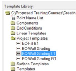
f. Select *EC-Wall Grading LT* and drag and drop it onto the end point of the back of sidewalk berm.
