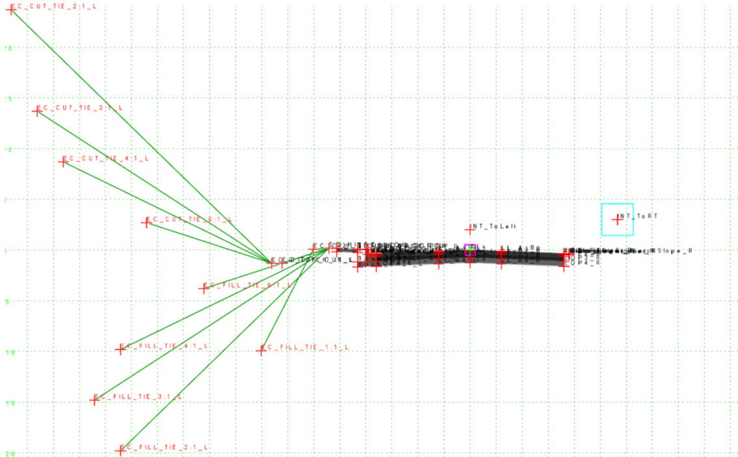
Add Corridor References for the *Ramp C* and *Ramp D* intersection. Intersection match line elements have been created for all intersections along the corridor.
