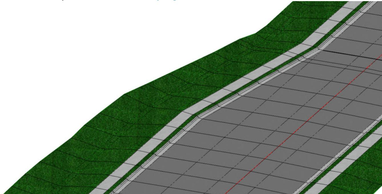
6. **Rotate** the 3D View to **Top** and note how the template drop changed direction and is now perpendicular the edge of pavement taper we defined as a **Secondary Alignment**.
