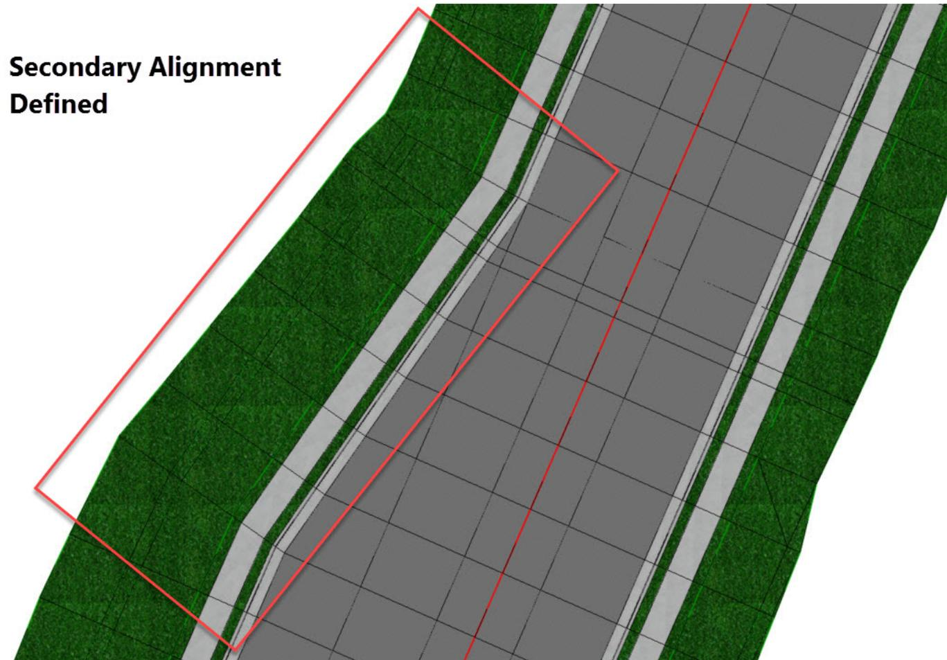
**Tip:** When secondary alignments are created, a graphical manipulator is drawn in the 2D view which enables you to graphically edit the secondary alignment.
