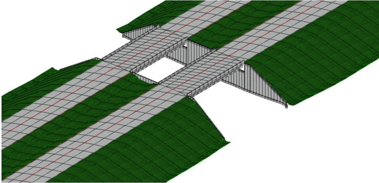
**Tip 1:** The bridges can be modeled in detail using Bentley OpenBridge Modeler. Or you can create a fairly accurate model of the bridge by creating a corridor and using a bridge template.
