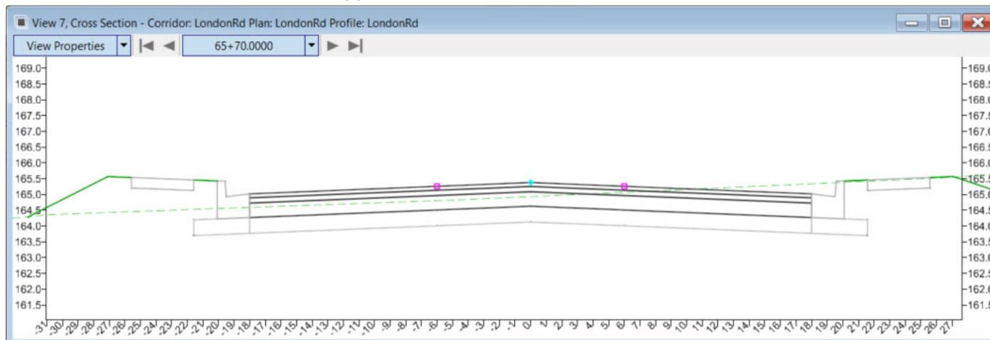
**Note:** This view window is showing dynamic cross sections extracted from the 3D model. All elements in the 3D model will appear in the cross section.
