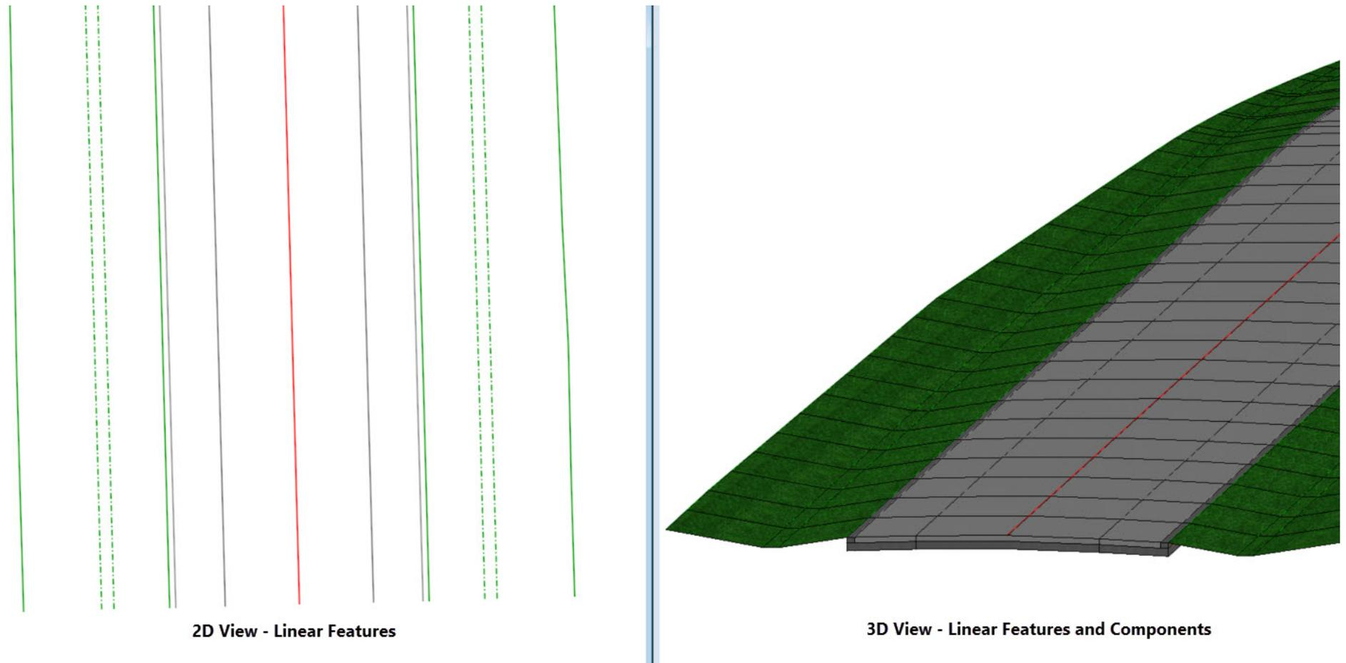
The 3D model can be displayed as components, linear features, a top surface mesh, or a bottom surface mesh. This is defined by the Corridor Feature Design assigned to the corridor when it is created. In our case the Corridor Feature Definition used was *Conceptual*.
