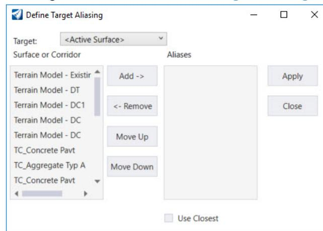
The left portion of the dialog displays a list of available terrains, corridors or features that you can target. The right portion of the dialog is where you define the *Aliases* (target terrains, corridors or features) and the processing order. When an end condition seeks a target it will start at the top of the *Aliases* list. If a target is not found the end condition will then work its way down the list until a target is found.
