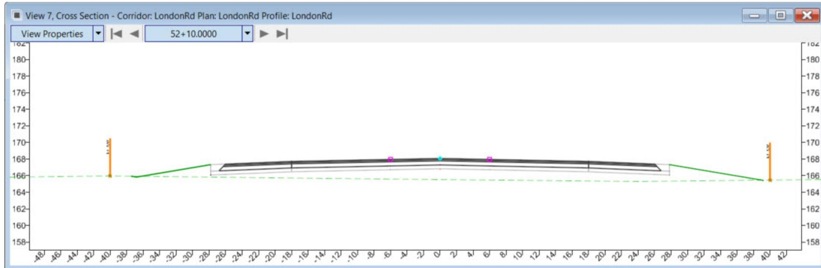
**TIP:** Right of way markers show up on the cross section automatically. This happens because the right of way file is attached as a reference and the right of way feature definition is configured to display a right of way marker on the cross sections.
