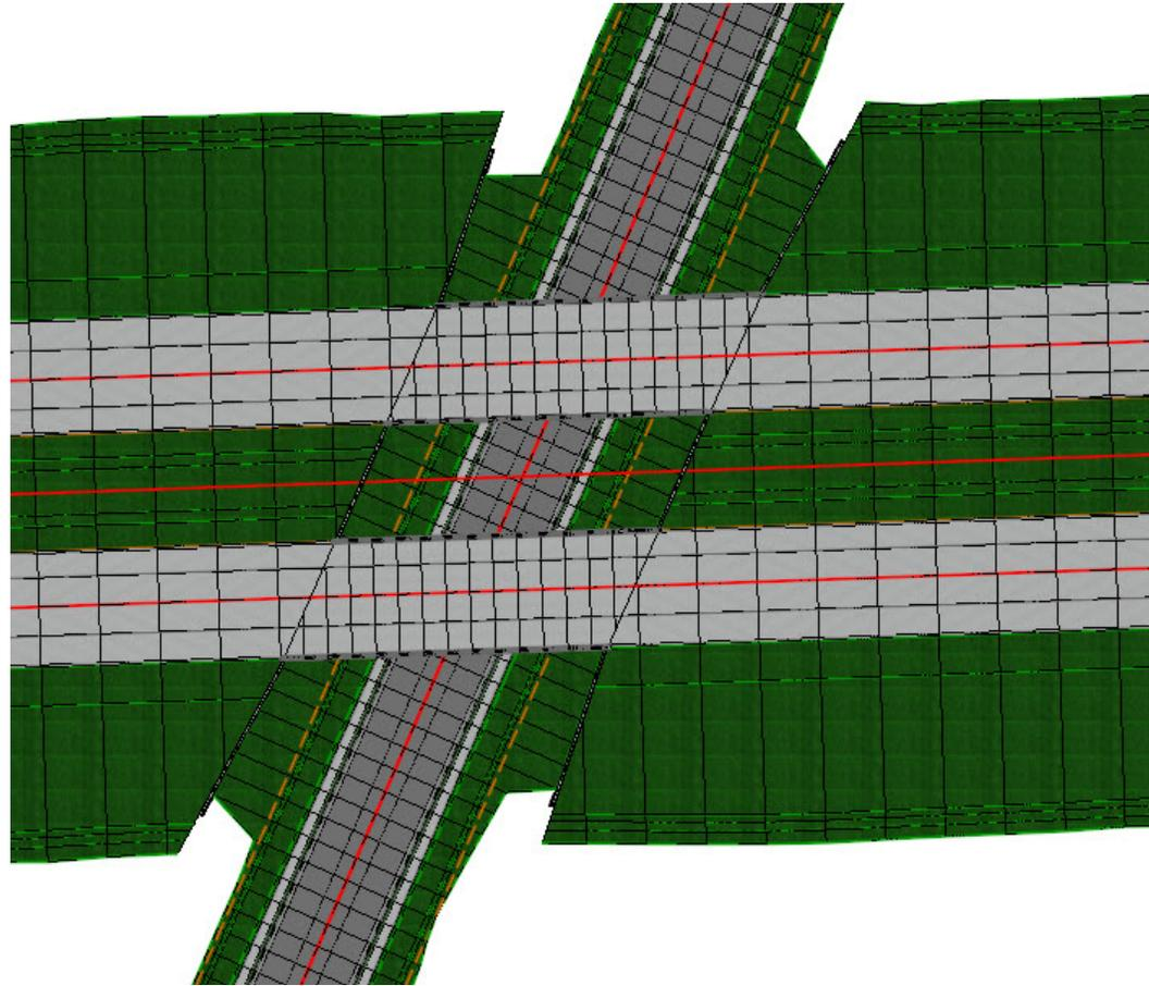
3. Create End Condition Exceptions to place a 8:1 ditch backslope on the left and right side of the corridor in the area of the walls. End Condition Exceptions are used to override the default template end conditions between a user defined station range.
