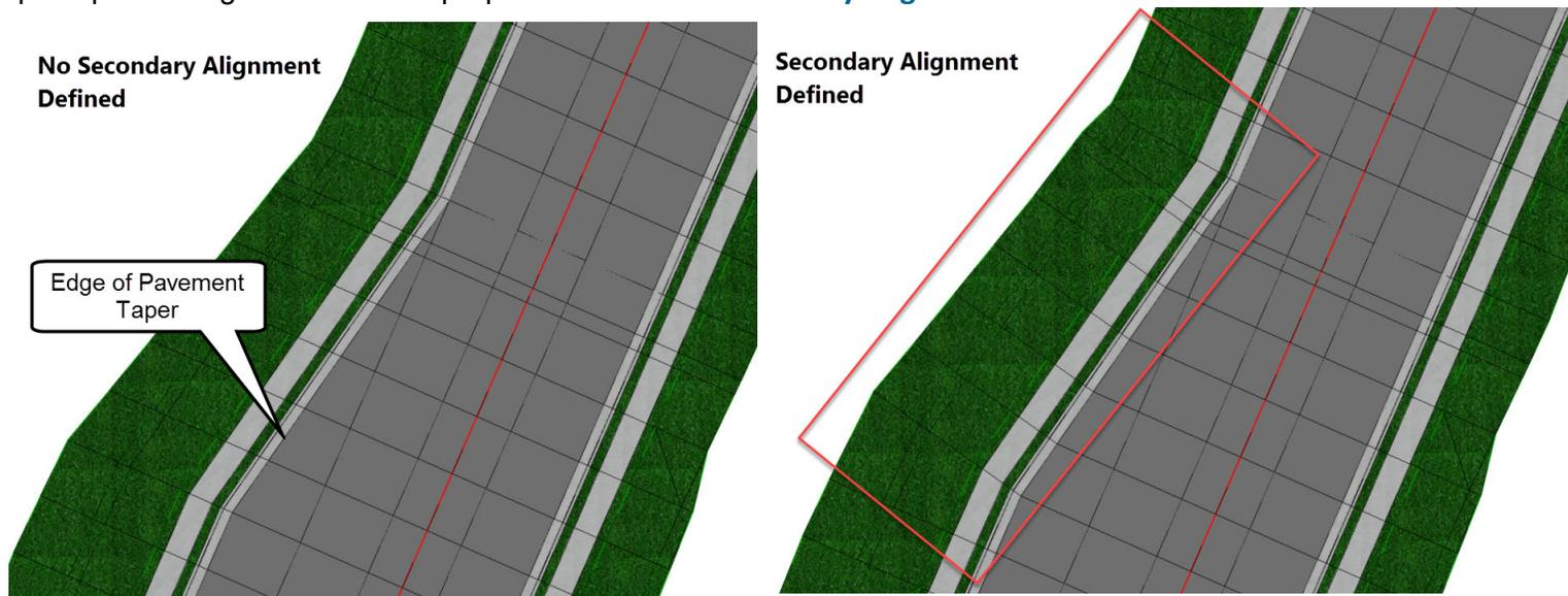
4. Add a **Secondary Alignment** to change the direction of the template processing to go perpendicular from the left edge of pavement taper.
