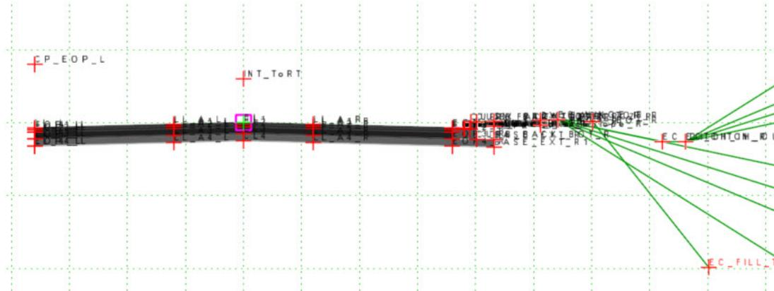
Notice there is a point named **CP\_EOP\_L**, this point will be used to control how the template widens horizontal to add the right turn lane.
