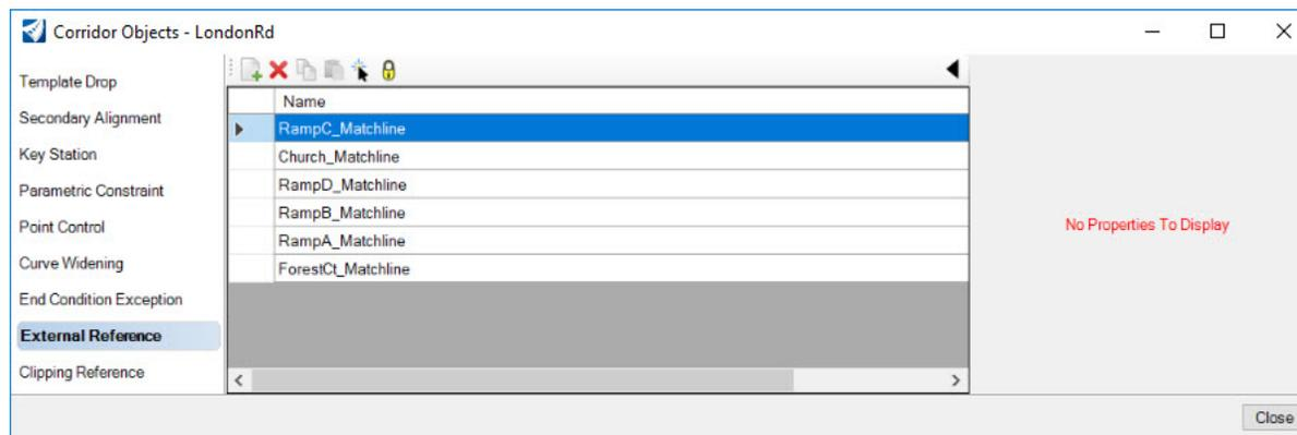
The *External Reference* portion of **Corridor Objects** shows you all the geometric elements that have been assigned as corridor reference. In our case, all of the intersection matchline elements that we added as corridor references. When you select a reference element in the list it will highlight in the 2D view.
