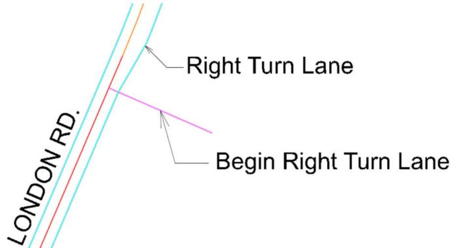
12. **Review** the 3D Model in the turn lane areas and note that the turn lane is not displayed. This is by design, in order for the turn lane to display you must add the edge of pavement as a corridor reference or create a point control to follow the edge of pavement.
